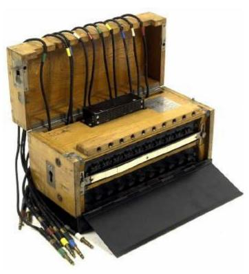
In 1877, Edwin Holmes, the operator of an electric burglar alarm business in Boston, installed the first telephone exchange. The first switchboard was connected to telephones in the offices of six businesses which had purchased alarms from Mr. Holmes. It served as a telephone system by day and a burglar alarm system by night.
